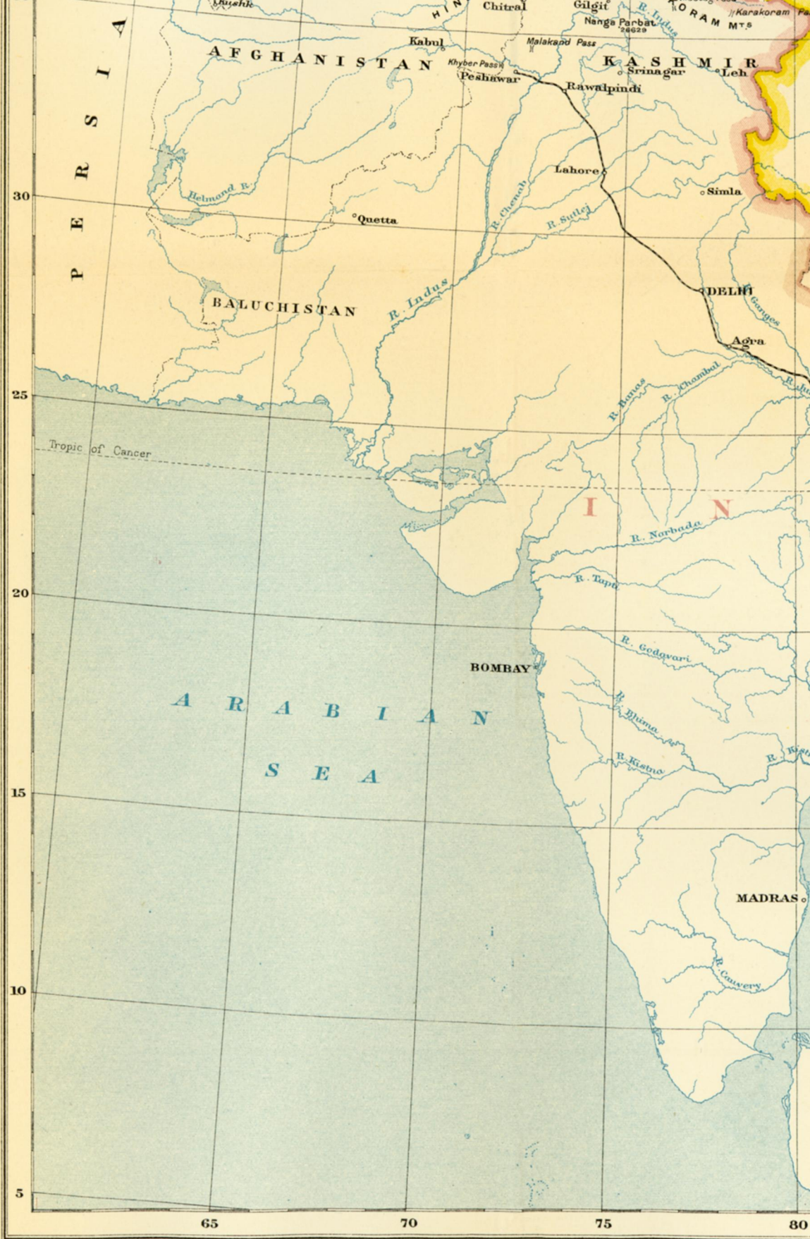
Modified Conical Projection with True Meridians and Errorless Parallels 10° & 34' 15"
